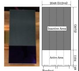
Figure 6: (left) Picture of 2k×1k CCD, (right) overview of 2k×1k CCD
